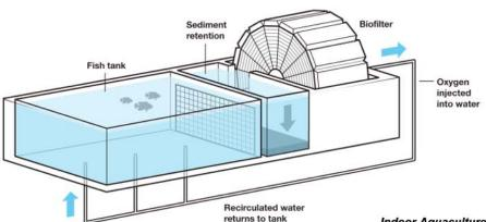
Indoor Aquaculture Water recirculates through biofilters packed with cleansing bacteria. Refreshed with an injection of oxygen, it returns to the tank. Collected sediment goes to a landfill.
